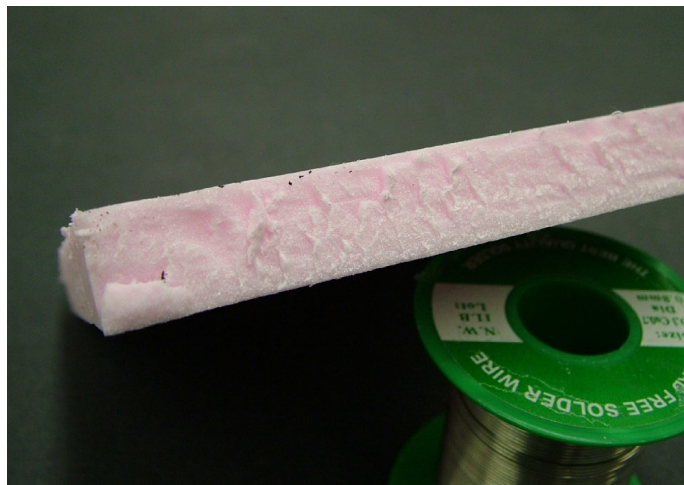
The edge of Styrofoam cut with a dull blade (I used a very dull blade to emphasize the damage done).
