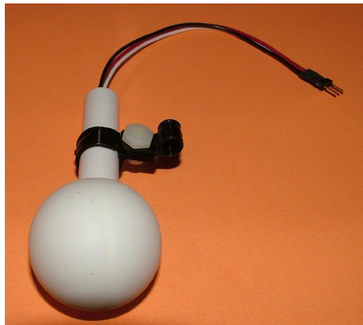
Figure 34. Two nylon wire clamps attach to the pillar of the light sensor. They connect to each other, back to back, with a nylon nut and bolt.
